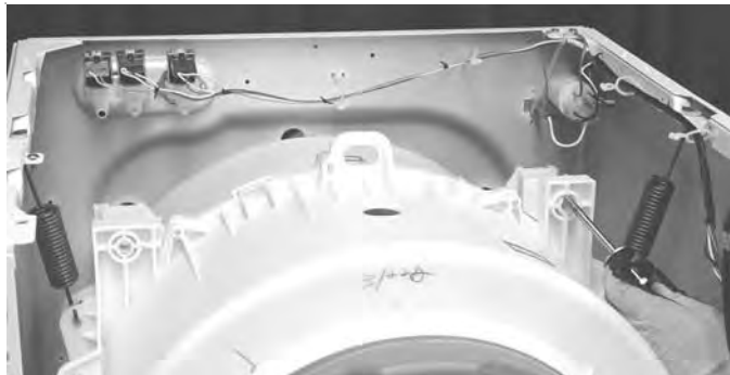
22. Reinstall Upper Counter Weight bolts to tub without weight in place. Use these as handles when lifting tub.
