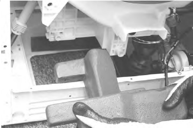
18. Remove remaining wire harnesses and hose from tub.
