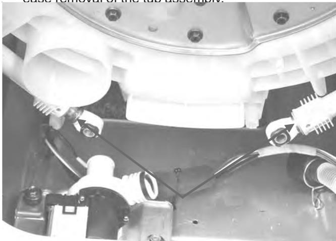
NOTE: The rear struts can be identified by the green sleeve.
