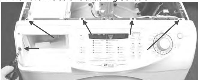
5. Roll Console down and lift away from washer.
