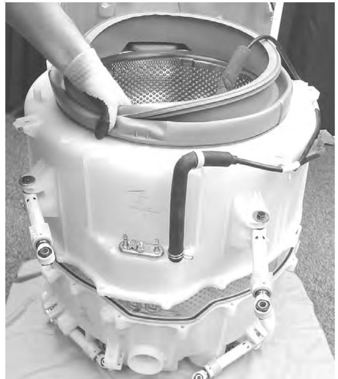
26. Tub Gasket can be replaced after tub halves are split.
