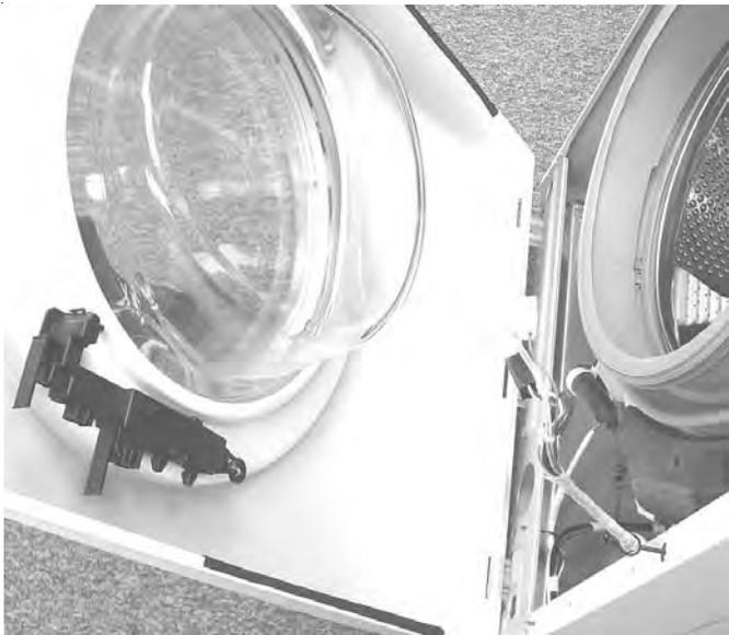
**NOTE:** When installing the boot align the index tabs on the boot with the screws on either side of the Fill Tube.
