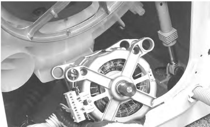
Normal resistance is approximately 3.0 $\Omega$  between any 2 pins (1,2 or 3) on motor connector.
