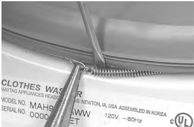
5. Pull the boot from the lip formed into the front opening.
