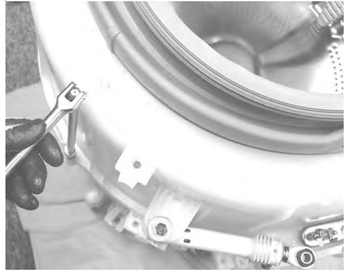
**NOTE:** Torque tub bolts to 6-11 ft. lbs.
