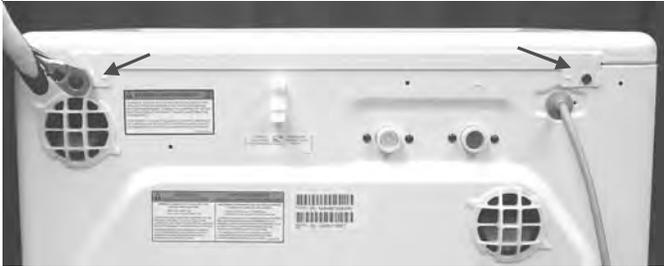
3. Slide Top Cover towards the rear to clear the screw head from flange on the bottom side of the Top Cover.
