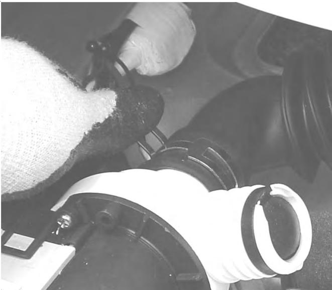
5. Remove wiring connector.
