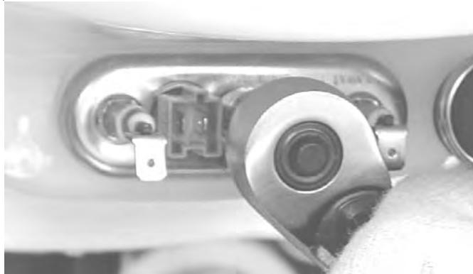
**NOTE:** Install Heater Element on top of metal bracket.
