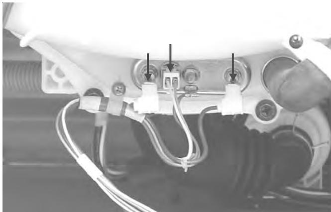
6. Loosen 10mm nut on Heater and remove Heater Element.
