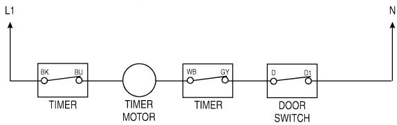
10. Timer Motor Circuit - Automatic dry cycle.
