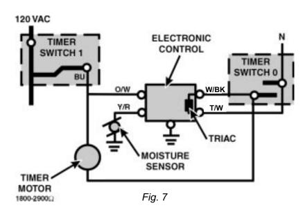
The electronic control looks at the input from the moisture sensor to see if the clothes are wet or dry. The moisture sensor will show continuity (short) if the clothes are wet and show **NO** continuity (open) if the clothes are dry.
