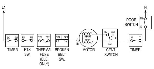
2. Drive Motor Circuit - RUNNING at speed
