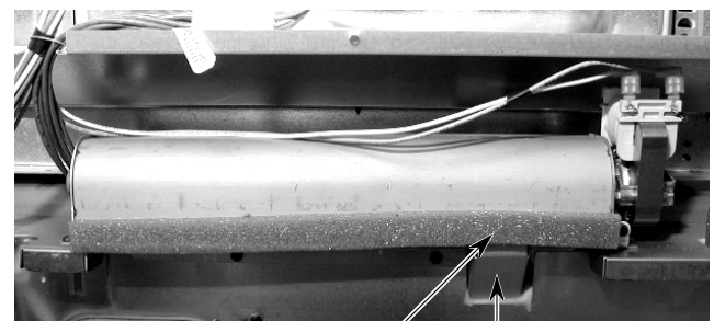
Foam Tape Over Air Duct Screw
