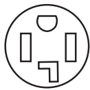
4-wire receptacle (14-30R)
