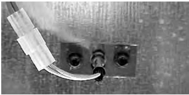
Oven sensor mounting screws
