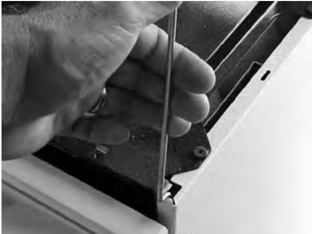
Coil element top lift and lock rod
