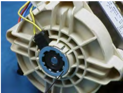
Tachometer mounted on the rear of the motor
