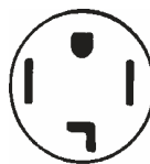
TYPICAL 4 CONDUCTOR RECEPTACLE
