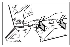
3) After releasing 4 hooks of control panel assembly, separate connectors from PWB assembly for disassembling control panel assembly.
