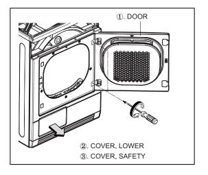
7) Disassemble 3 screws.
