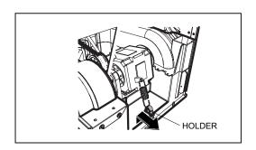
15) Disassemble Blower cover by unscrewing 2 screws. Note: Make sure that hook is properly fit after assembling Cover Base Wrong assembly will cause abnormal noise.
