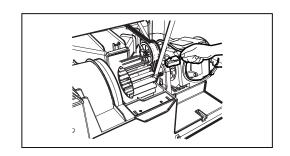
19) Disassemble Duct by unscrewing.
