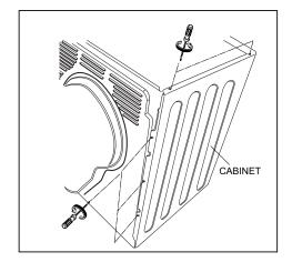
12) Disassemble Body frame by unscrewing 4 screws.
