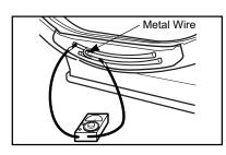
With metal tape attached to Sensor tips, CN1 3 - CN1 2 resistance is less than  $10\Omega$ ?
