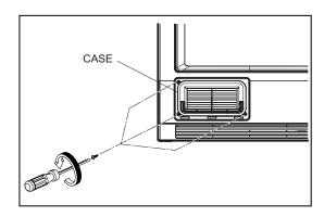
8) Disassemble the case with a Philips driver by releasing hook.
