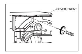
29) Disassemble Cover Front by pulling the top area out.
