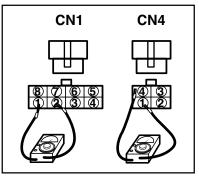
With CN1(RED4), CN4(WH4) disconnected from Controller, check
