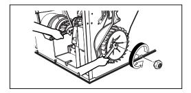
21) Disassemble moisture Sensor by detaching Inner Connector harness and unscrewing 3 screws.
