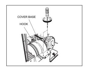
16) Disassemble Motor Supporter from Base by rotating after unscrewing 2 screws.
