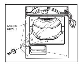
11) Disassemble cabinet by unscrewing 2 at the top and 3 at the rear (left and right are the same).
