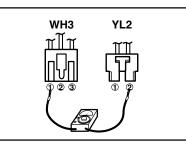
With door closed, check voltage of connector WH3③ and YL3① which are pulled out from controller in advance. The voltage range is between AC 215~245V?
