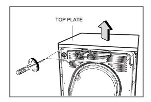
2) After pulling drawer assembly out, unscrew 1 screw.
