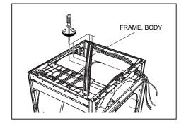
13) Disassemble Harness by unscrewing 2 Earth screws and disassemble connectors.
