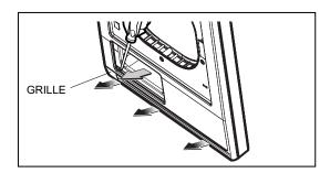
10) Disassemble the cabinet cover by removing 9 screws.
