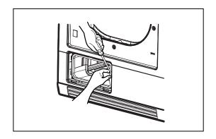
9) Disassemble grille by releasing 3 hooks.
