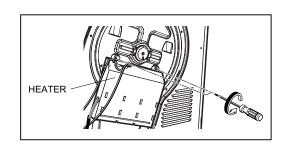
26) Disassemble Frame Top by unscrewing 4 screws. (Left and right are same)
