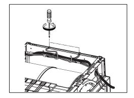
14) Disassemble Holder and Spring by pressing down and pulling the low hook of holder.
