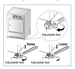
When pushing down the opposite corners of the machine, the machine should not move. (Please, check both directions) If machine rocks when pushing the machine top plate diagonally, adjust the feet again.
