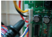
typical PCB Ground CN1#3(Black)
