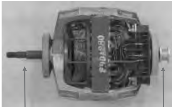
Fan connection axis
