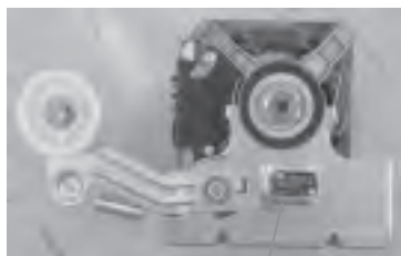
Damaged belt - switch lid pressed by the sp
