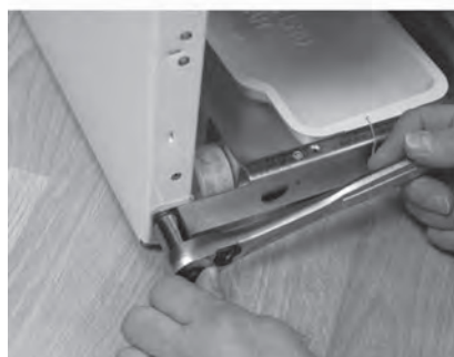
6. Remove 1/2" bolts on left and right hand sides.
