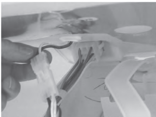
4. Disconnect wire harnesses.
