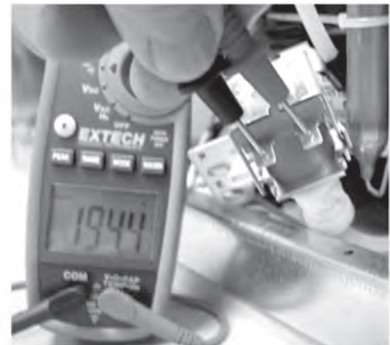
Connect meter leads across the valve terminals.
