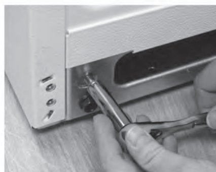
4. Remove 3/8" bolts on left and right hand sides.
