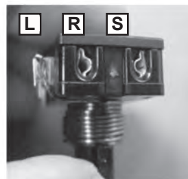
Terminal Identification L - Line R- Run S- Start
