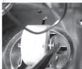
1. Fold the locking tab down to allow the axle to be removed from the roller and bracket.
