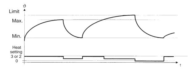
If the temperature limit is exceeded, all heaters are switched off. The heater is not switched on again until the temperature has dropped to  $\upsilon$  min. If the temperature does not drop below the temperature limit within 10x30 sec., the drying process is terminated and an "Overheating" error message (extra dry LED) is output.
