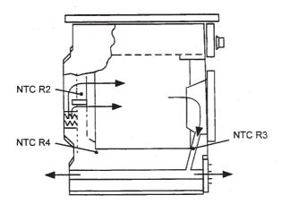
NTC R3 is situated in the ring insert under the door and measures the exhaust-air temperature.
