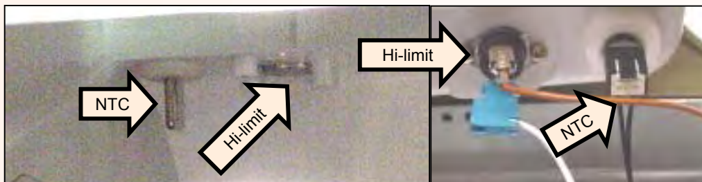
NTC R3 & B19 Hi-limit in bottom of front shield
